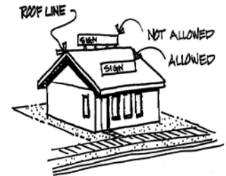
Roof Line and Roof Sign
